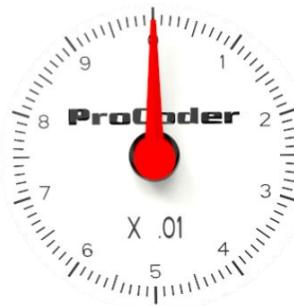
A typical ProCoder sweep hand contains 10 large ticks numbered 0-9. Between each large tick, there are 9 small ticks numbered .1 - .9. Depending on the size and meter type, a multiplier will also be present and located below the red hand. Let's demonstrate how to read the sweep hand.
