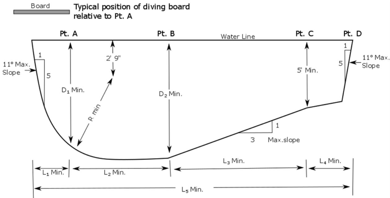
Note: L<sub>4</sub> is a minimum dimension to allow sufficient length opposite the board. This may of course be lengthened to form the shallow portion of the pool.
